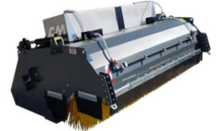
Sweeping bucket, with bucket collector and ø800 mm polypropylene brushes, for high power operating machine, with the purpose of cleaning streets, squares, and outdoor floors of any type. It is produced with widths ranging between 200 cm and 300 cm.
