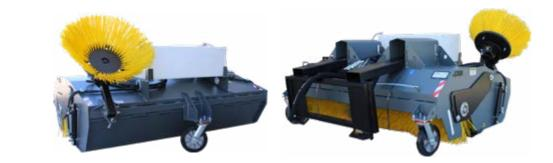
With front bucket collector and polypropylene brushes, equipped with three revolving support wheels, it is particularly indicated to clean fine particles and is recommended on middle-heavy applications/works. It is produced in 9 models with different useful widths ranging between 105 cm and 250 cm.
